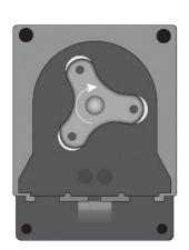
Position the roller at 7h05, turning it in the direction of the circular arrow.
