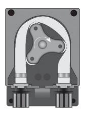
Position the roller at 7h15, turning it in the direction of the circular arrow.
