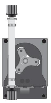
Insert the left connector into the relative housing and pass the hose under the roller's guide. Turn the roller in the direction of the circular arrow, simultaneously accompanying the hose into the pump's head, until the right connector is reached.
